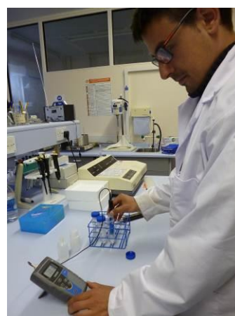
Figure 4. Soil water analysis by ion selective electrode.
