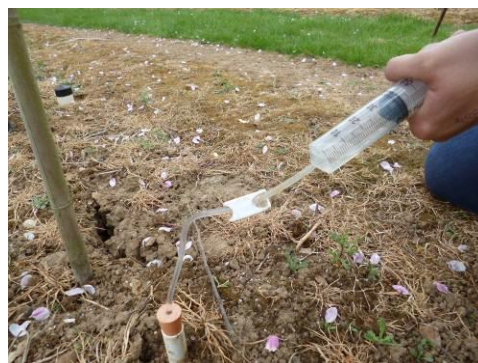
Figure 3. Soil water sampling from a suction cup lysimeter at 60 cm soil depth
